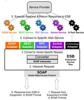
Figure 5: The architecture of the proposed ESB
