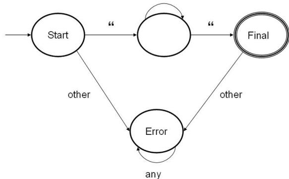
Fig 3: Finite Automata for String Values
